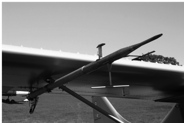
Fig. 7 FTI pitot boom installed below the Trial right wing.
